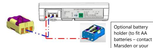
4. Place the housing back inside the indicator, and close the battery housing cover.
