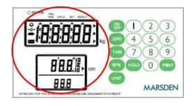
The scale will first test all of the display segments.
