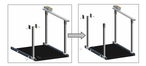
Step 5. With handrails assembled, attach no.13 (bracket for indicator) using no.6 (screw)
