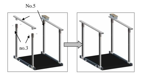
Step 6. For M-652, assemble cross bar (SS-8444) with two screws (M8-1.25P\*45).
