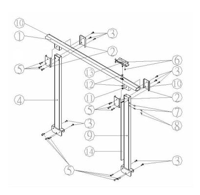
Fix no.2 (fixing plate) on no.9 (pole with wiring duct) with no.3 (socket screw) and no.5 (screw nut).
