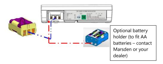
4. Place the housing back in the back of the indicator, and close the battery housing cover.
