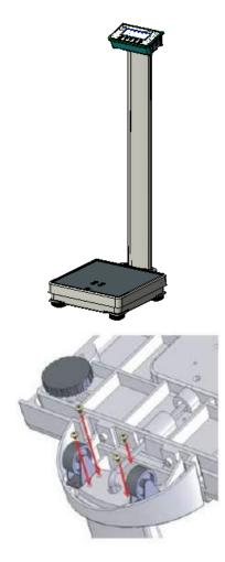
Position the column so that it is resting on the base, ensuring all wiring from the base to the indicator is safely tucked inside the column housing.
