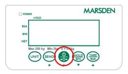
Press the ON/ZERO/OFF button firmly.
