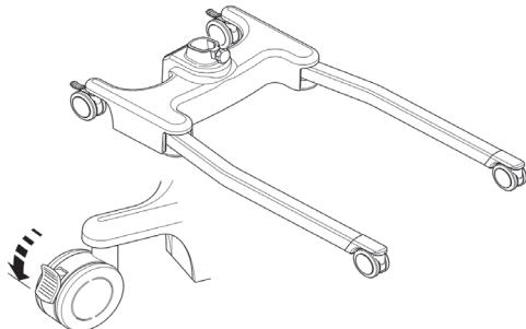
2. Fit the mast and boom assembly into the chassis socket
