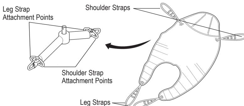
**6-point spreader bar.** Example of 6-point spreader bar sling with loop attachments.
