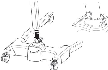
3. Tighten the mast assembly with the mast-locking device, which is located at the front of the chassis.
