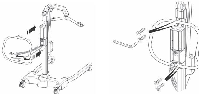
6. Fit power pack to the lift and make sure the latch holding the pack in place is fully engaged. “Click” in place.
