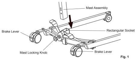
**4.** When the mast is fully engaged within the socket, turn the mast locking knob (Fig. 1) clockwise, until fully tightened.
